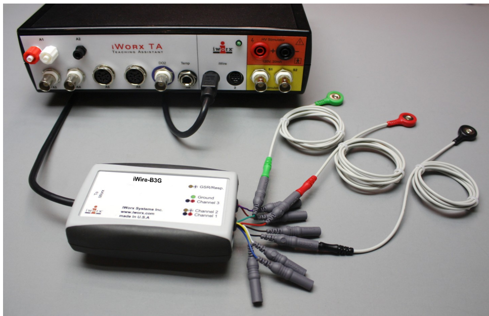
Figure HC-6-S1: A iWire-B3G ECG cable with 3 lead wires connected to an iWorx IXTA.
