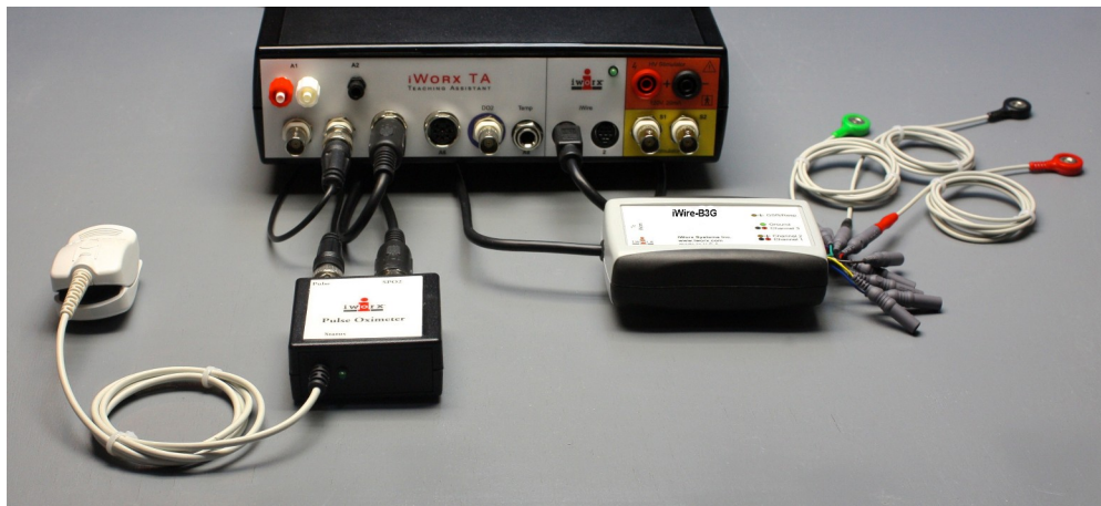
Figure HC-6-S3: A PO2-100 pulse oximeter connected to an IXTA.
